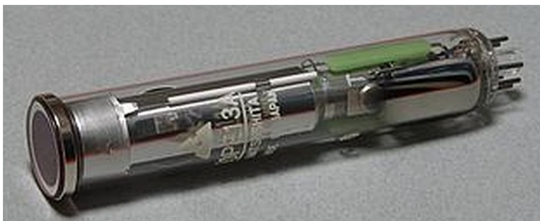
Video camerabuis, circa 1960, later vervangen door plumbicon
